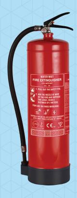
Ceasefire's watermist-based portable extinguisher is powered by Watermist. Once the system is triggered, a specially designed rotor within the mist generator mixes air and water in a pre-set proportion to generate Watermist. The mist is then propelled at the fire through a specially designed nozzle with a throw of 10 feet. The mist then quickly blankets the flames and brings down the temperature to below combustion levels.
