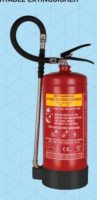
In commercial kitchens, the liberal use of fire and the presence of combustible substances make it easy for a fire to flare up. Designed to fight kitchen oil and fat fires, Ceasefire's Wet Chemical-based Fire Extinguisher uses an environmentally friendly foaming agent that blankets the flames, cuts down the supply of oxygen and cools the oil to below self-ignition point.
